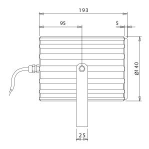
1) Drill the mounting location holes for the loudspeaker inline with the "U" bracket (2 holes 30 millimetres apart) in the surface where the loudspeaker is going to be located. It is not necessary to use the central mounting hole in the bracket unless the loudspeaker is used with a pole mount clamp.
