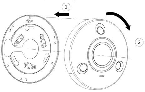
Find the gap on the camera body; align it with the "TOP" on the corresponding quick mounting board, rotate the camera body clockwise to complete installation.
